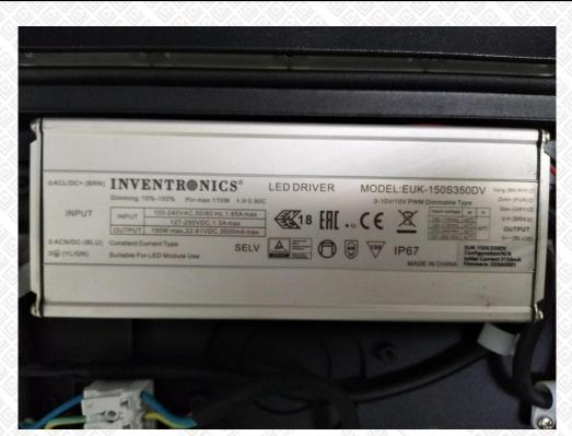
Figure 6 (Label of the LED driver)
